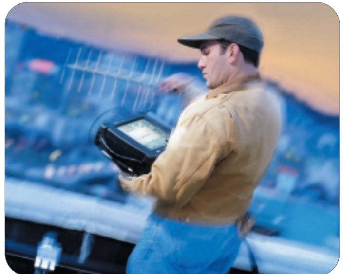
► Figure 15. Using the directional beam antenna and the signal strength measurement.
